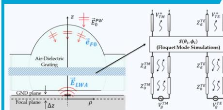
The CFO theoretical framework, developed during this ERC, in combination with a Spectral field representation of the leaky waves and grating geometries for a complete analysis of these lens antennas enabling a fast optimization of its radiation properties.
