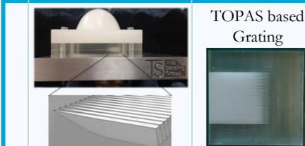
**Key idea:** Using the new leaky-wave antenna integrated with a non-periodic gratings, we have shown enhanced the steering properties in low-permittivity lenses in combination with planar focal plane arrays
