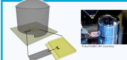
**Key idea:** The combination of a quartz-cavity leaky wave exciting a shallow silicon lens with and a beam-lead transitions to GaAs GaAs front-ends.
