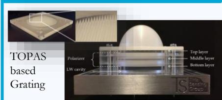
**Key idea:** leaky wave antennas radiate most of the energy below the critical angle. This fact enables the embedding of air-dielectric gratings (non-uniform dielectrics) into the lens for tuning it radiating properties such as generation of circular polarization
