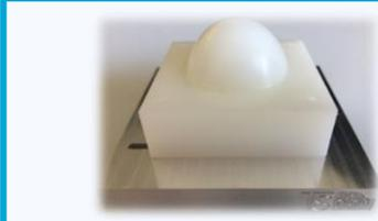
**Key idea:** Compact, low cost and wide-band integrated lens leaky wave antennas based on very low dielectric permittivity. It can be scaled in directivity easily and to higher frequencies
